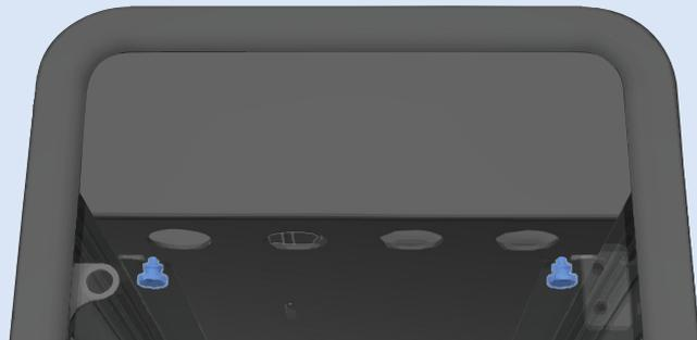
Security screws located underneath the removable AC tray on both sides.
