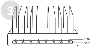
Plug the USB-C to USB-C charging cables that come with the charging dock into the charging ports.
