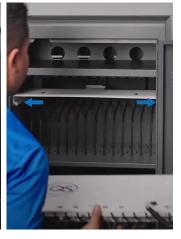
Optional: Use the Philips head screws to secure the bracket to the sides of the cart (Blue Arrows.)
