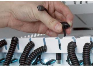
2: To replace cables, unplug the port end and safely 3: Once all the cables that need to be replaced are feed them through the bracket. Installing cables is reversed. Feed the cable through the brackets, then plug the ends into ports.
