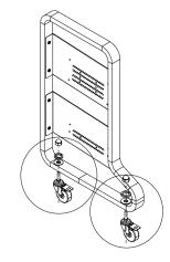
1: Engage the brake lock on each caster (T20) if it is not locked already. Using the supplied wrench (J10), secure 2 casters (T20) to each side panel (L12), (M13) of the cart using 1 flat washer (F6), 1 spring washer (E5), and 1 nut cap (D4) on each caster.
