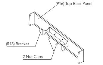
2: To install the power cable wrap bracket, locate the 2 PEM studs on the back of the top back panel piece (P16) and remove the nut caps from the studs using the socket wrench (K11). Position the bracket (R18) onto the studs and then tighten the 2 nut caps back onto the studs to secure the bracket in place.
