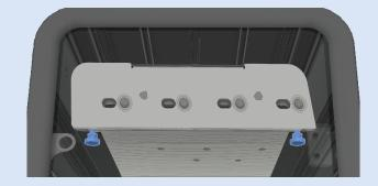
Use the wrench to remove the bolts on both sides of the Quick-Sense USB-C module to remove it.
